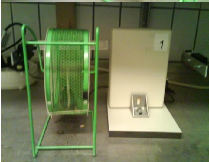
Figure 1. Computerized running wheels used for the 30-min or 10-min exercise sessions and for registration of number of revolutions/session from which was derived distance run.
